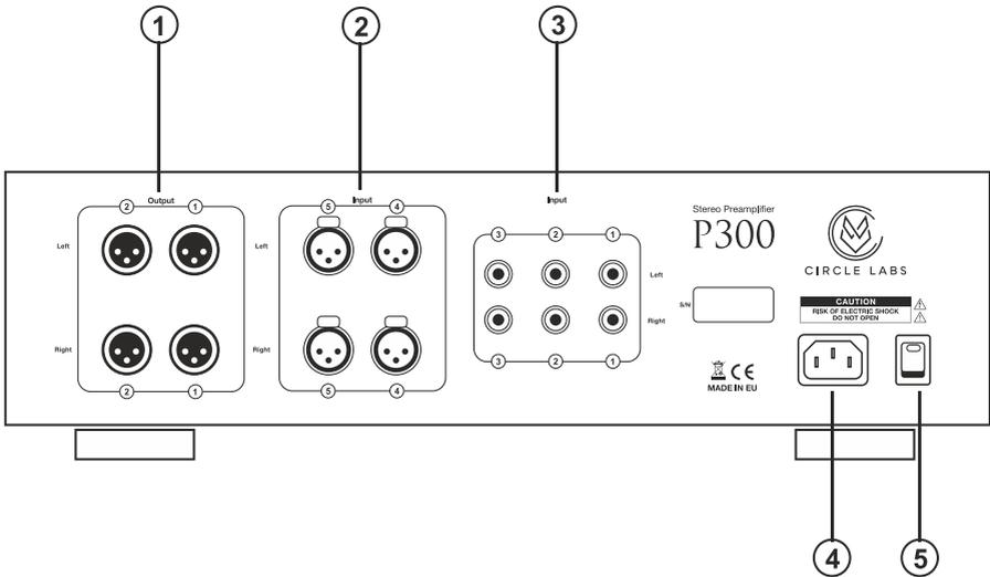
1. Balanced XLR outputs (output impedance 15Ω)
